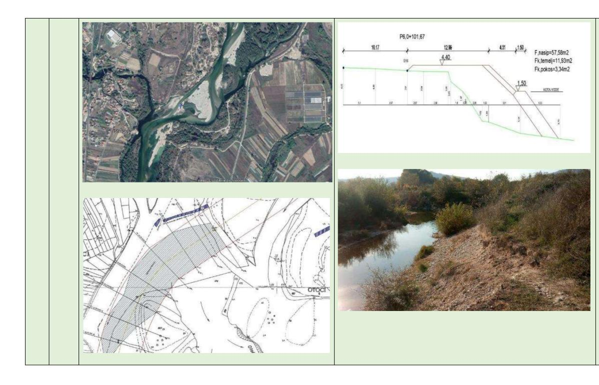
No additional excavation is necessary from the river bed. On critical parts, excavated flood deposit from riverbed will be used for backfilling of eroded bank. No additional excavation of eroded banks is required.
