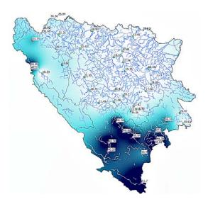
Figure 6: Average surface runoff (outflow) in BiH (expressed in l/s/km²), according to the discharges registered in the profiles of surface watercourses (Source of data for creation of the map: Framework Water Management Plan of BiH, 1994)
